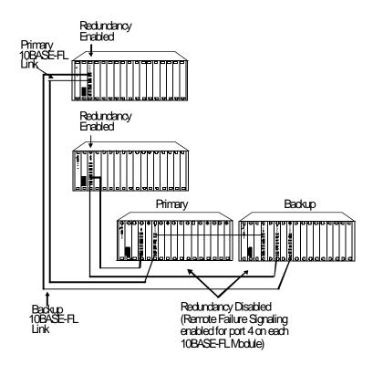
Figure 2-10. Redundant Fiber Backbone Configuration
